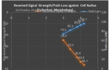
Fig .8: The effects of the power received, Path loss and cell radii on signal coverage in suburban morphology
