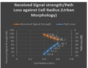
Fig.7: The effects of the power received in base station, Path loss and cell radii on signal coverage in urban morphology
