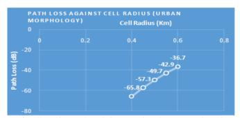
Fig.1: The effects of cell radius and path loss on signal coverage in urban morphology From Fig.1, it noticed that cell radius and path loss have common relationship. The cell radius increase with increase in path loss, and also the cell radius decrease with decrease in pathloss
